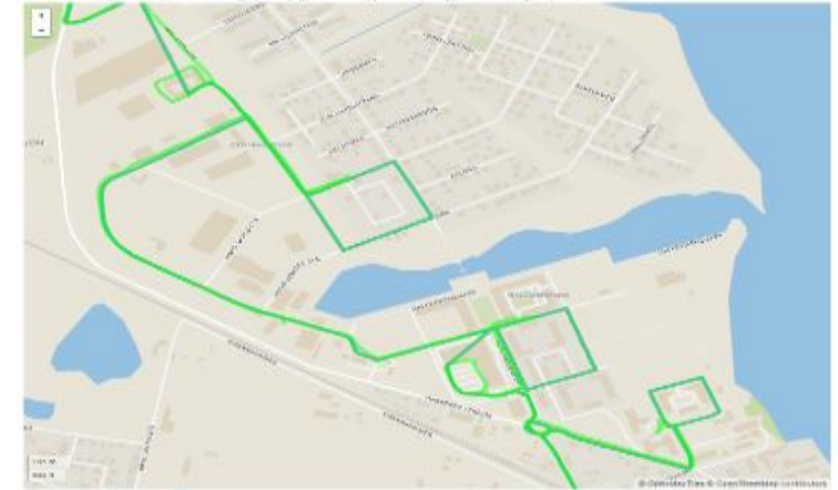
Ghost loops – driver took a straight way but map matching generated loops
